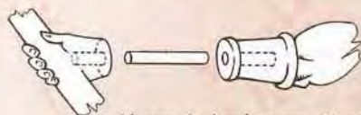
Above: A simple representation of the pinning process Below: A pin vice drill
